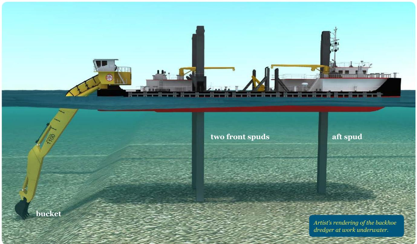
out of the water, a part of the weight of the dredger is now transferred via the spuds to the seabed, resulting in an increase in anchoring. This is sufficient to deliver the required resistance to the digging forces. Secure anchoring makes the BHD less sensitive to waves, currents or the wake of passing vessels.
