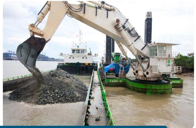
*One advantage of a BHD is its ability to dredge a wide range of subsoils, clayey soils, stones, even materials containing boulders or debris.*
