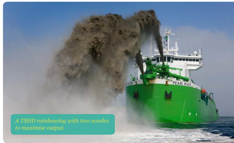
*A TSHD rainbowing with two nozzles to maximise output.*
