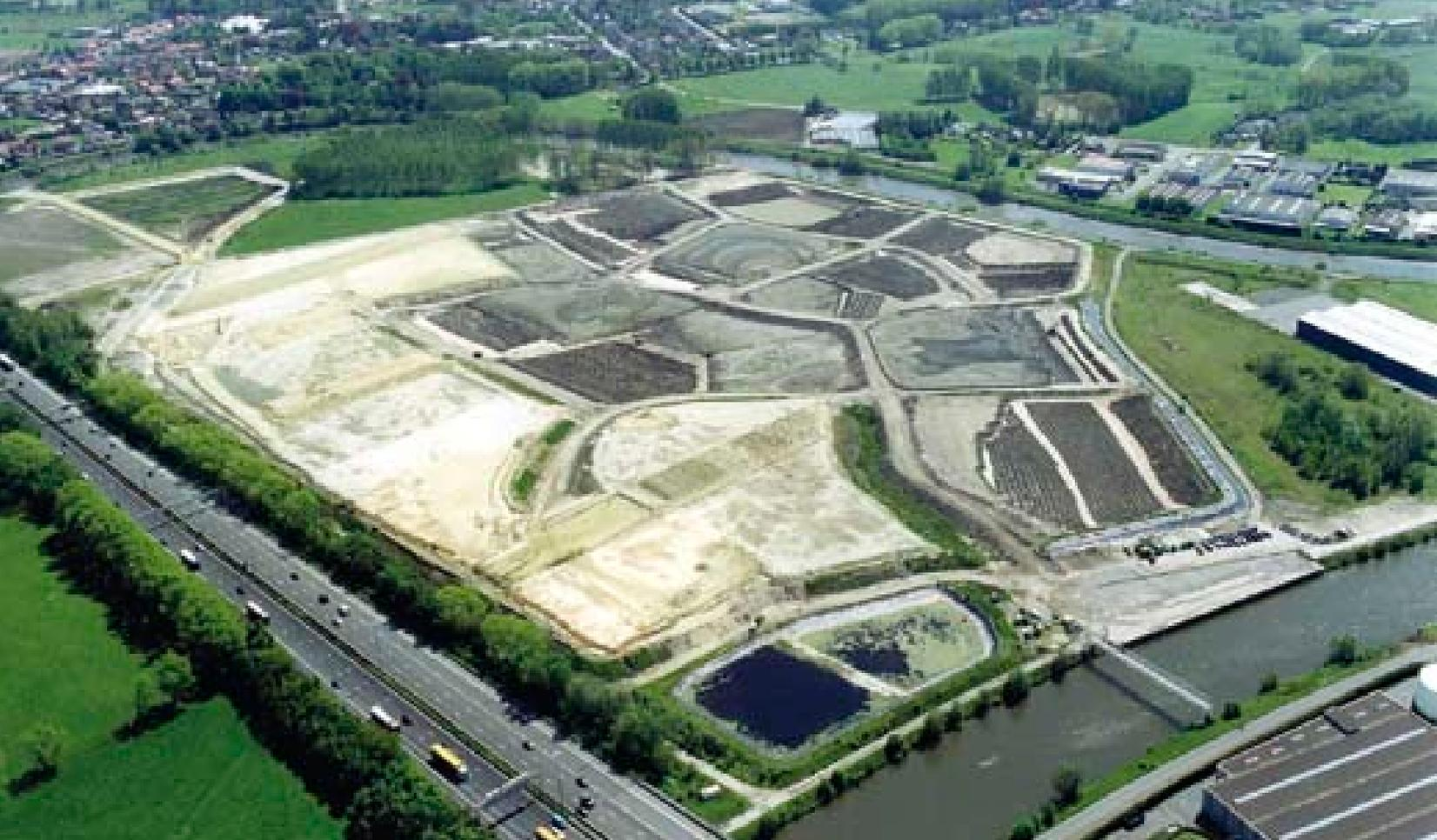
Figure 1. Aerial view of the Fasiver site in the process of being treated with millions of tonnes of clean dredged material.
