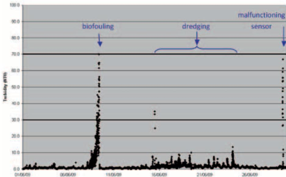
Figure 7. Turbidity values measured at a telemetry buoy during June 2009.
