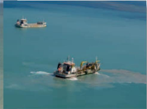
Figure 8. Above, turbidity plume created during dredging by the TSHD De Bougainville.
