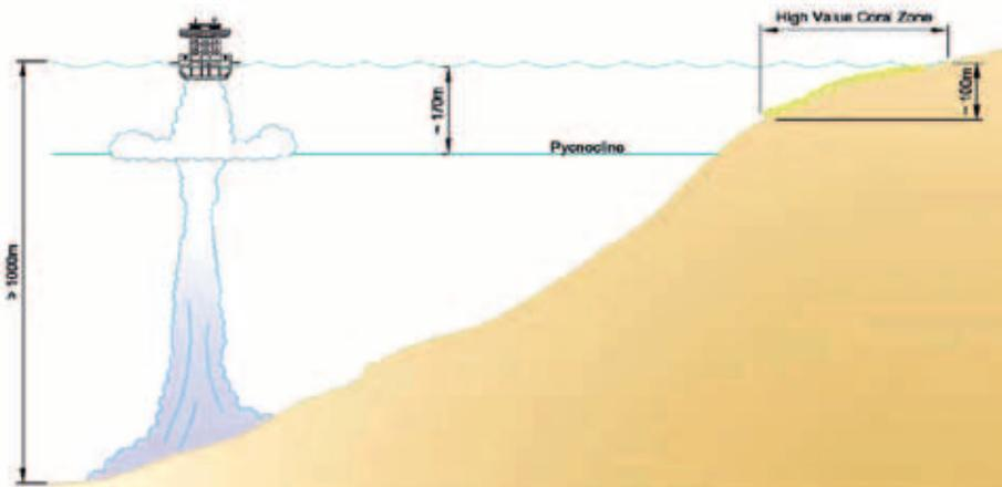
Figure 4. Possible effect of pycnocline on sediment settlement at the disposal site (source: EIA).
