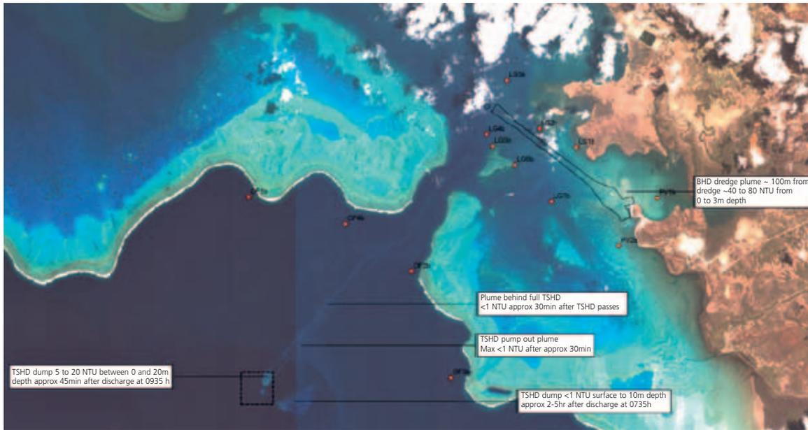
Figure 11. Satellite image taken on 21/09/2008 with indication of the NTU of the different plumes (source: KBR and Koniambo Nickel SAS).
