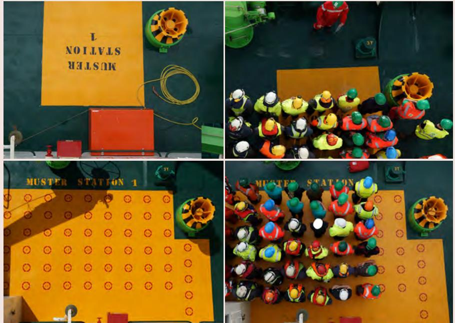
Top left and right images show the muster station before painting numbered circles on deck. The bottom two images show the muster station after it has been enhanced.
