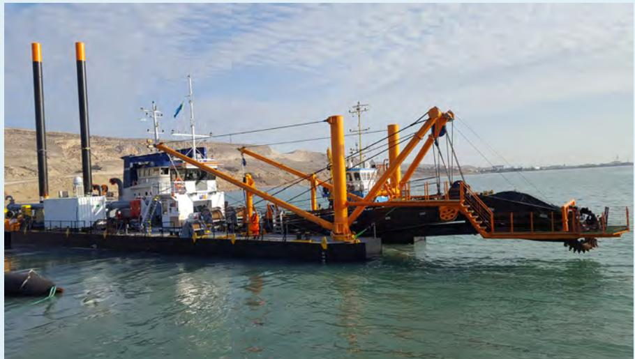
The light weight cutter platform ensures employees can work safely while replacing cutter teeth and conducting maintenance.
