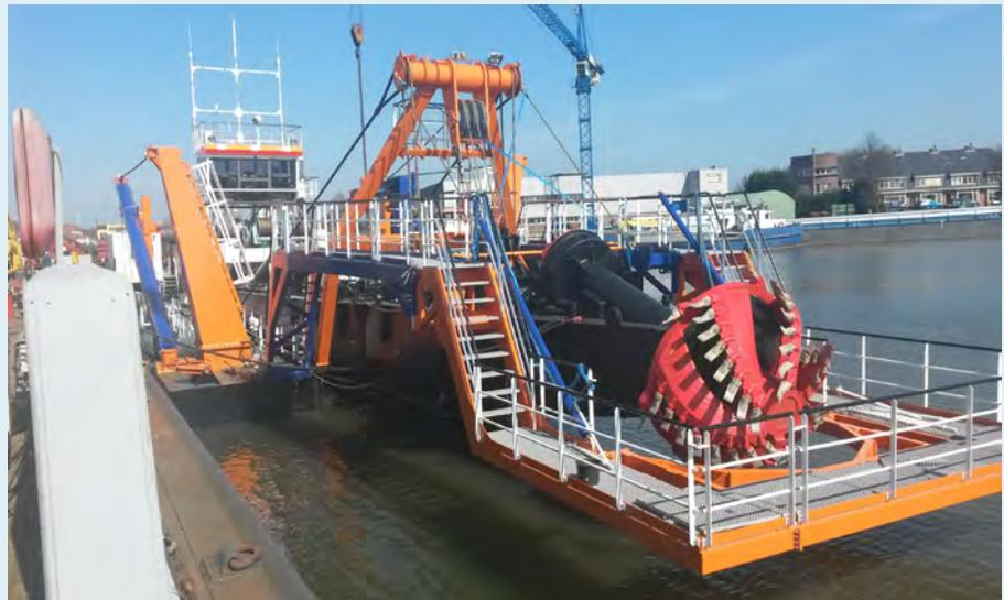
Royal IHC developed various innovative safety features on a CSD; Biesbosch features a cutter platform that improves accessibility around the cutterhead.
