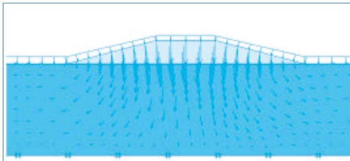
Figure 11. Deformation pattern in finite element software.
