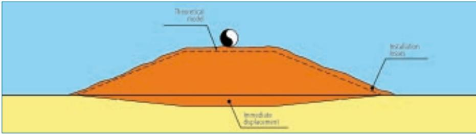
Figure 8. The total required volume of rock for one support can be determined when the theoretical rock volume required to install the support, the installation losses during operations and the immediate displacements of the seabed are considered.
