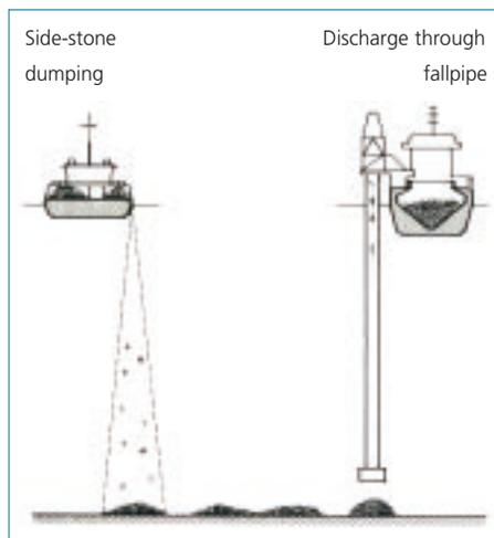
Figure 5. Schematic drawing of two methods of rock placement.
