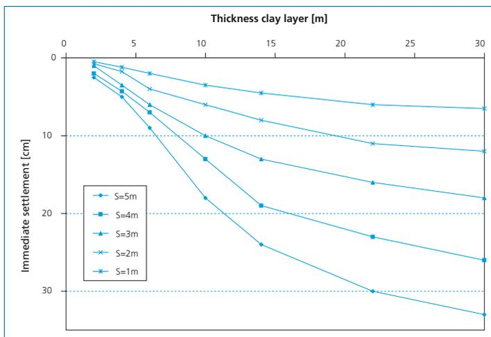
Figure 12. Immediate deformations in clay for deformation modulus  $M = 2\text{MPa}$ . Each line represents a different support height S.
