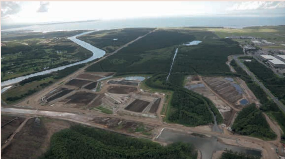
Figure 1. Aerial view of the works at the Second Parallel Runway for Brisbane Airport, Australia. Thirteen million m<sup>3</sup> of sand will be placed.
