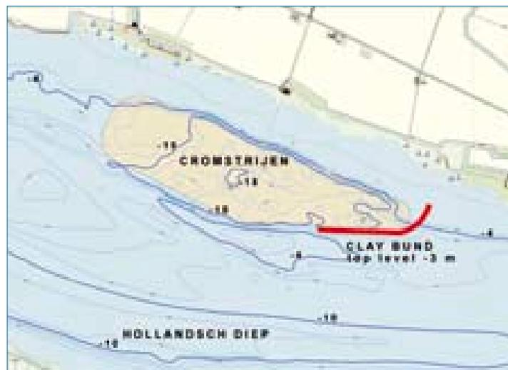
Figure 5. Schematic drawing of the former borrow pit “Cromstrijen”, with a capacity of 10 Mm<sup>3</sup>, which was provided with an underwater bund at the upper boundary.
