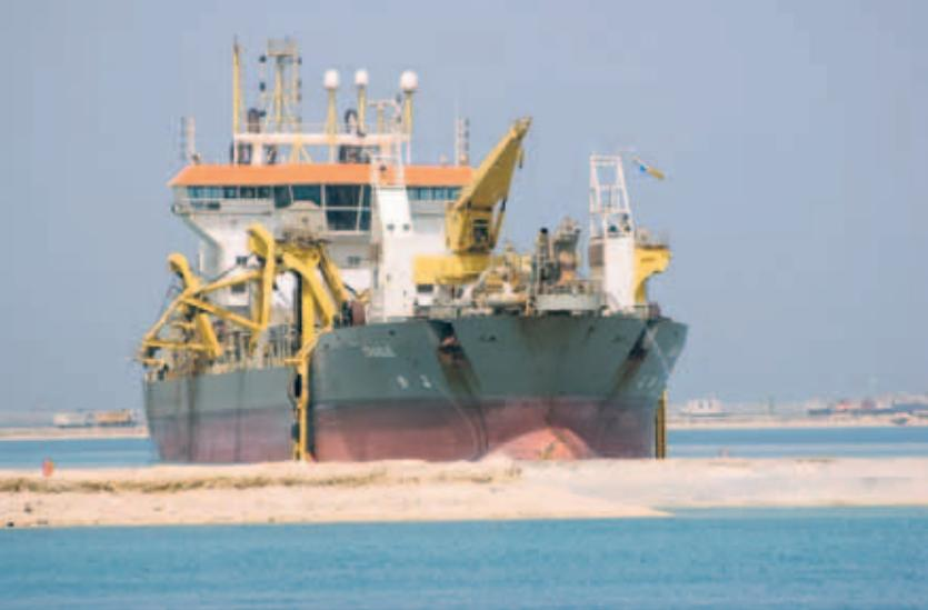
Figure 3. One of the trailers, the TSHD Oranje, working at Ras Laffan Port Expansion project.
