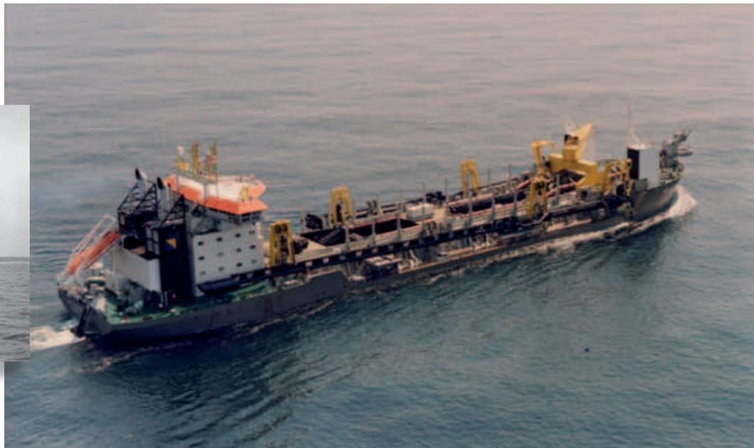
Figure 4. The second TSHD *W.D. Fairway* (built in 1996 and lengthened in 2002).
