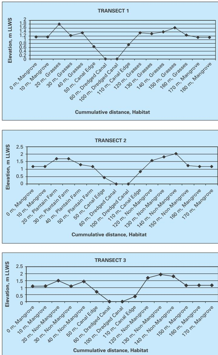
Figure 5. Microtopographic changes in a dredged material disposal area.
