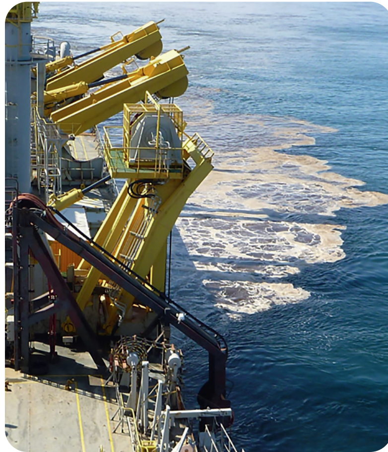
Effect of environmental valve: valve off (above) and valve active (opposite page).
